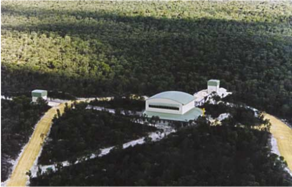
Figure 10 Aerial photo of the AIGO site 80 km north of Perth. Two 80 m arms are visible extending from the central laboratory. The site benefits from minimal seismic interference from human activity, and unspoiled natural bushland abounding in biodiversity.
