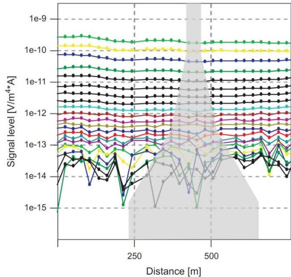
**Figure 3. Trapezoid filters for the stacking from the raw to the average data**
