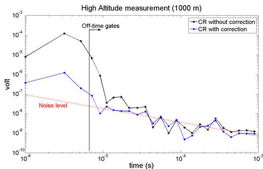
**Figure 2. Removing of the Coil Response at High Altitude. The black curve is the measured data while the blue curve is the CR corrected curve.**
