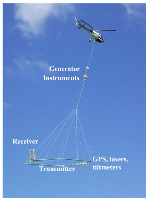
**Figure 1. The SkyTEM101 system in the air. The receiver coil is integrated into the tail of the system. The altitude is measured by two duplicated lasers and the pitch and roll by duplicated tiltmeters.**
