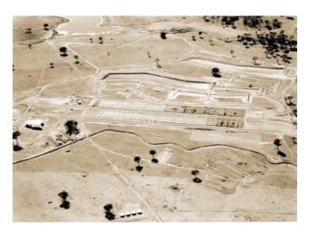
**Figure 6.** Aerial view of the cattle research (feedlot) facility, 'Tullimba' Armidale NSW. The facility has 1000-head capacity with 16 pens equipped for individual feed-intake measurement. Purpose-built drainage and sediment ponds designed for feedlot waste management studies. Contours and waste water collection allow for total containment of all effluent.
