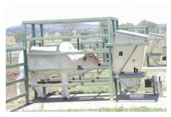
**Figure 8.** Animal at 'Tullimba' individual feed intake recorder. Note feed hopper (a) and cleaning door (b).
