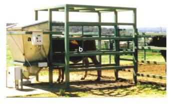
Figure 9. Side view of 'Tullimba' individual feed intake recorder showing computer (a) and infrared beam emitter (b).
