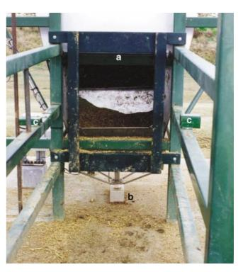
**Figure 10.** Animal's eye view of individual feed intake recorder showing animal identity reader antenna (a), load cell (b), and infrared beam emitter and reflector (c).
