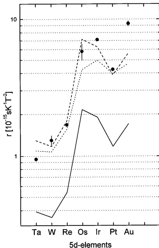
**Fig. 5.** Overall systematics (intrinsic SLR rates  $r_\infty$  versus impurity  $Z$ ) for dilute 5d series impurities in Fe. The experimental points were obtained in this work or by Beck *et al.* (1996) and Bobek *et al.* (1993). The solid curve represents the calculations of Akai (1988), the dashed curve gives Akai's results scaled upwards by a factor of 3.3, and the dotted curve is the sum of Akai's values and an estimated virtual spin-wave contribution (cf. Masuda *et al.* 1974).
