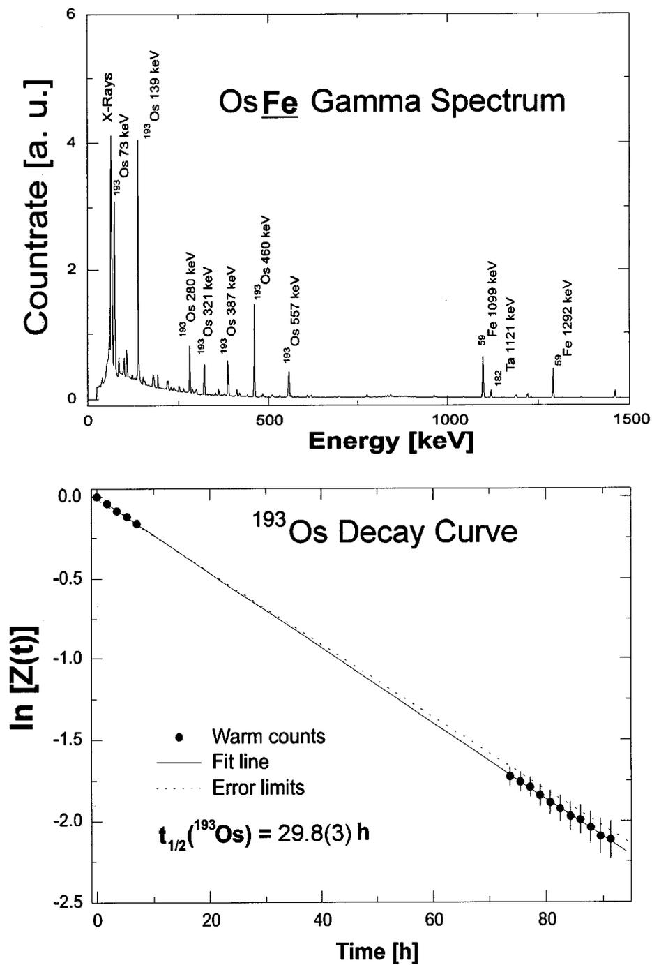
**Fig. 1.** Gamma-ray spectrum of a  $^{193}\text{OsFe}$  sample (upper part), showing the strong 139 keV line used for TCON data analysis. The lower part shows our redetermination of the decay half-life of  $^{193}\text{Os}$  using the 'warm counts' from the sample.
