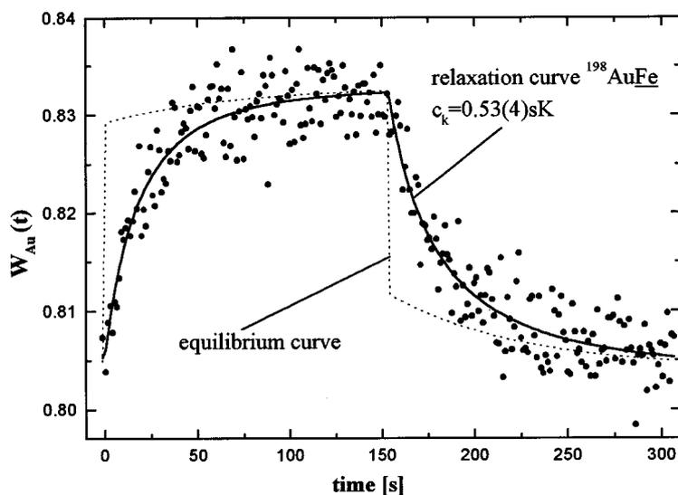
**Fig. 3.** Relaxation curve for  $^{198}\text{AuFe}$ , similar to Fig. 2. Note that the lattice temperature follows nearly a step function, although a small ‘tail’ due to temperature-dependent heat capacities and warming of the surrounding materials by the heat pulse is still present.
