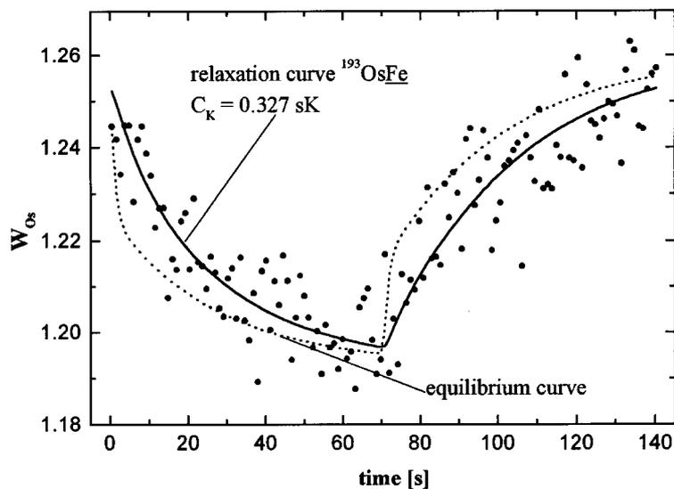
**Fig. 2.** Relaxation curve for  $^{193}\text{OsFe}$ . The dotted curve shows the lattice temperature  $T_L(t)$  as determined by the fast nuclear thermometer. The solid curve is the fit to the multi-exponential relaxation function taking the momentary temperatures into account.
