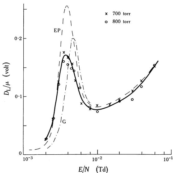
Fig. 1.—Ratio  $D_L/\mu$  for electrons in argon at 90 K. The bold curve shows the present experimental result. The other curves have been calculated (see text) from the cross sections of:
