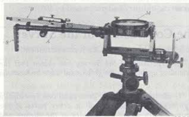
Figure 8. The Thalen-Tiberg magnetometer - the least sensitive instrument used.
