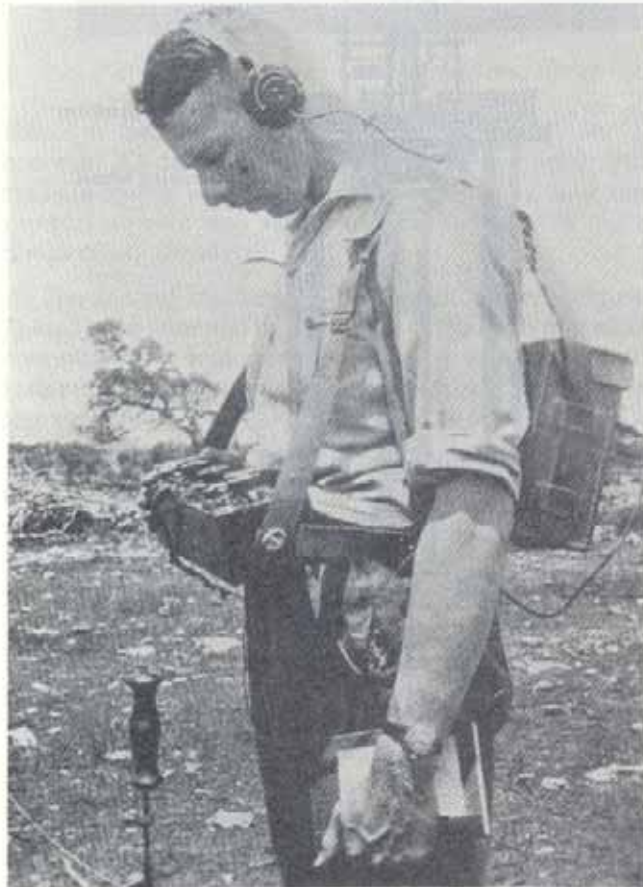
Figure 2. Ratiometer in use with amplifier on the operators back.
