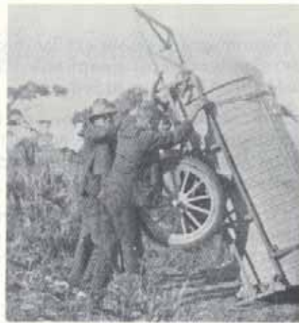
Figure 6. Transportation and erection of Oertling torsion balance.
