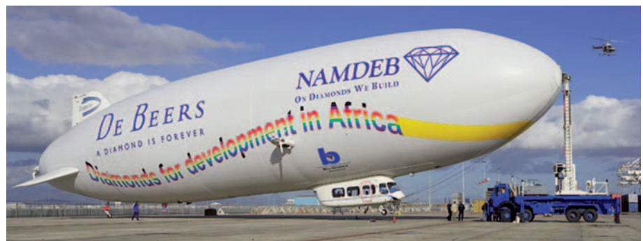
Fig. 1. The Zeppelin NT-07 airship used for the test program in Germany and Botswana. It is seen mounted on a mast truck, which holds the airship secure when on the ground. The engines on the side and end of the hull can also be seen; these provide vector thrust control at low flight speeds.
