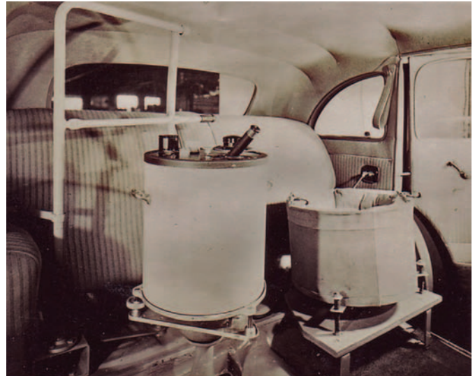
Fig. 10. 'Gravimeter mounted on tripod in reading position. The instrument determines variations in gravity of the order of 1 part in 30,000,000' (Rayner 1946, p. 2).
