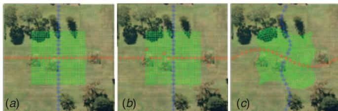
**Fig. 1.** (a) An ideal regular grid layout. Source locations are in red, receiver locations in blue, and the resulting common midpoints in green. (b) The same layout after the source positions have been moved to avoid some trees. (c) A new layout made possible by recent developments in processing software. The locations do not need to conform to a grid or to any particular pattern. Provided the locations vary reasonably smoothly, the result is uniform coverage.
