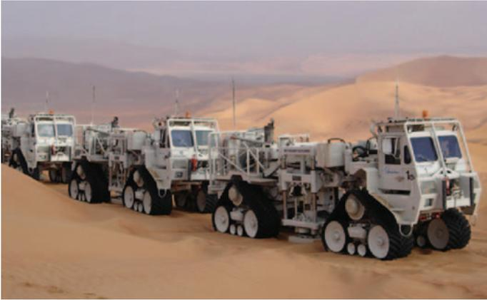
**Fig. 9.** Rubber tracked DX80 80 000 lb vibrators. (Image courtesy of WesternGeco.)
