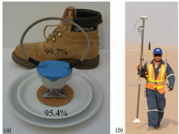
**Fig. 2.** (a) Accuracy of SBAS positioning. The probability that the measured position of an object will be within its true position is shown for objects of varied size relative to the size of a sensor. For example: boot or plate 99.7%, coaster 68%, saucer 95.4%. (b) UniQ positioning-with-layout equipment in use. A GPS antenna is at the top of the pole and the RFID system at the bottom. (Image courtesy of WesternGeco.)
