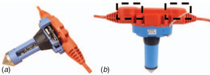
**Fig. 3.** Sercel DSU3 3-component MEMS sensor (left) and DSU3GPS sensor (right). The latter includes a pair of GPS antennas, highlighted by the dashed black boxes, to record the position and orientation of the sensor. (Image courtesy of Sercel.)
