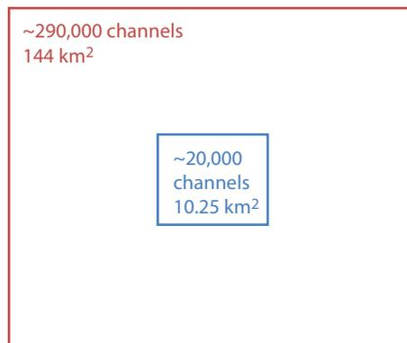
**Fig. 8.** Areas and channels for surveys in Kuwait during 2004 (10.25 km<sup>2</sup>, 20 000 channels) and one proposed in 2010 (144 km<sup>2</sup>, 290 000 channels).
