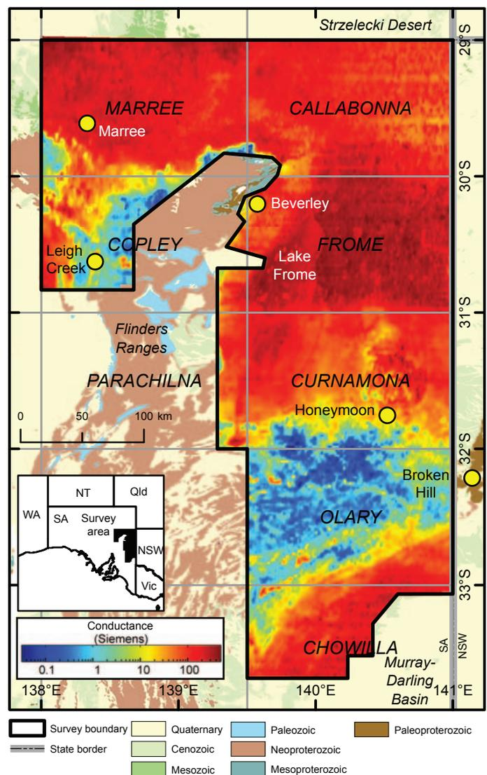
**Fig. 1.** The Frome Survey area highlighted with an image of the estimated conductance to 200m depth and 1:250 000 map sheet names. Geoscience Australia funded 5000 m line spacing across the entire survey and a large infill area at 2500 m line spacing. The Department of Manufacturing, Innovation, Trade, Resources and Energy South Australia (DMITRE) and a consortium led by Callabonna Uranium Ltd. funded infill areas at 2500 m line spacing.
