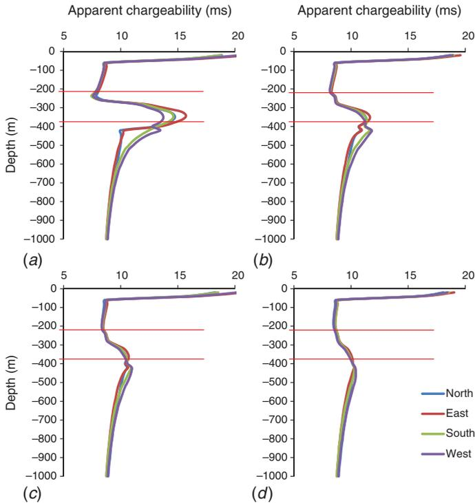
**Fig. 3.** Vertical profiles of apparent chargeability from drillholes with (a) 25, (b) 50, (c) 75, and (d) 100 m displacement between the deployed Axial Gradient Directional Array and the target. Red horizon lines denote the vertical position of the target.
