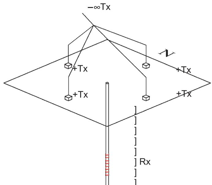
**Fig. 2.** Schematic diagram of the Axial Gradient Directional Array.
