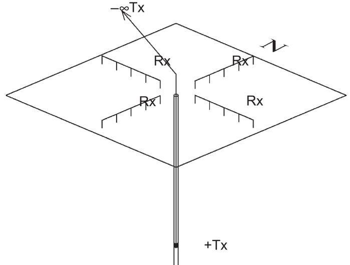
**Fig. 4.** Schematic diagram of the Radial Array. Note that only four potential arrays (Rx) are pictured, but the array may include many more at a specified angular interval.
