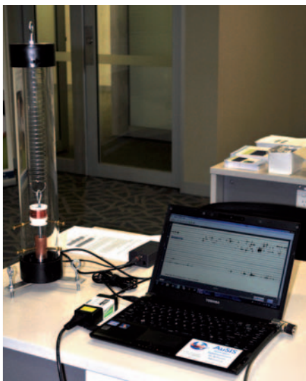
Fig. 4. Slinky Seismometer developed by Boise State University and its output to a laptop (see http://cgiss.boisestate.edu/bsu-network/ ).
