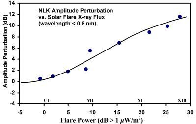
Figure 3 Solar flare induced amplitude enhancement in NLK signal as function of peak solar flare X-ray flux in dB (relative to  $1 \mu W/m^2$ ) in the 0.1-0.8 nm band.
