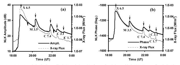
Figure 2 (a, b) Variation in the amplitude (a) and phase (b) of NLK signal along with the GOES X-ray flux during the solar flares on 6 December 2006.
