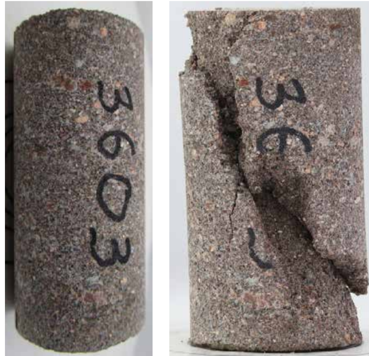
Sample photos pre- and post-test for test 3603. Sandstone from Munta 1, 1983.71 – 1983.81 m depth (GA sample ID 20212578). Core plug is 25.45 x 53 mm.
