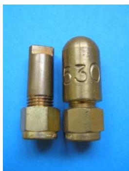
**Figure 1.** Differences between a New Zealand (left) and Australian sheep permeation tube.
