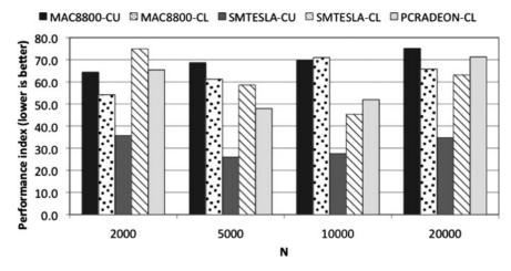
**Figure 1** Performance index [measured execution time scaled by (*N*/1000)<sup>3/2</sup>] for the NBODY1 code using CUDA (MAC8800-CU, SMTESLA-CU) and OpenCL (MAC8800-CL, SMTESLA-CL, PCRADEON-CL) kernels to directly calculate the interparticle forces, for varying system sizes. Lower performance index is better.
