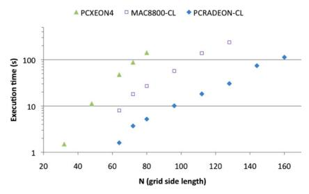
Figure 4 Measured execution time for the brute-force evaluation of equation (2) on a  $N^5$ -cell grid for a quad-core Xeon processor (PCXEON4) and OpenCL (MAC8800-CL, PCRADEON-CL) kernels. Lower execution time is better.
