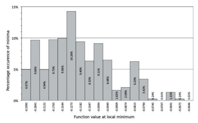
**Figure 3** Distribution of minima found by GSL simplex routine for minimisation of equation (1), with starting values in the range [-10, 10] for (x, y). Results based on executing code  $10^4$  times. The actual global minimum is only found in  $\sim 5\%$  of runs.
