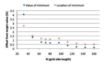
**Figure 5** Convergence of BFM minimisation to the value and location of a global minimum of equation (2) as a function of the grid side length *N*. The value offset is expressed as a percentage of the target minimum value; the position offset as a percentage of the diagonal length of the 5-dimensional parameter space.
