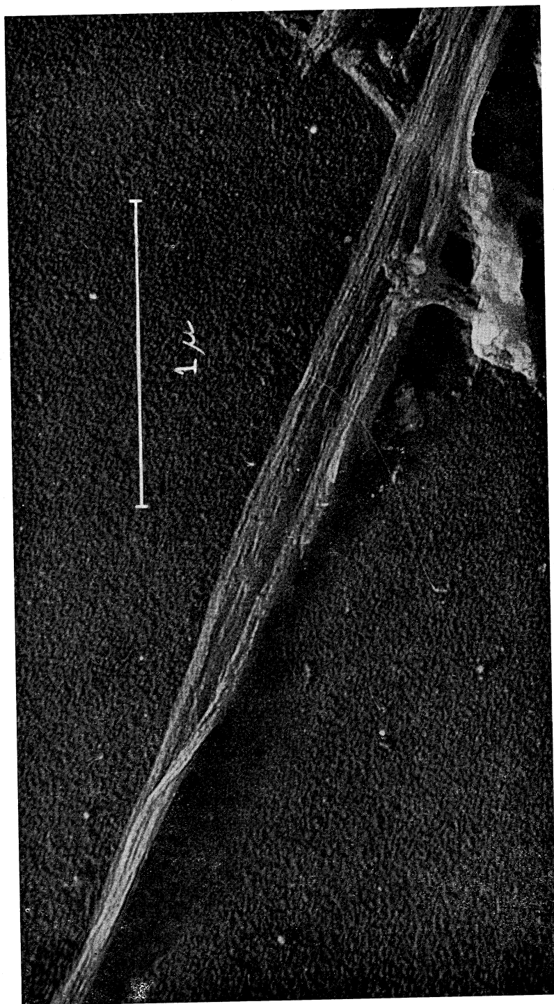
Fibrillar fragment from silk subjected to prolonged digestion with trypsin. Note fine, parallel fibrils. Shadowed with uranium.
