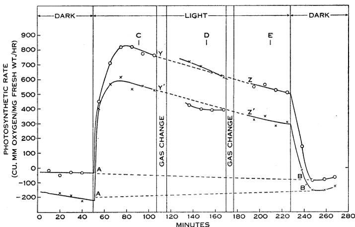
Fig. 6.—*Funaria hygrometrica*: Comparable samples initially in nitrogen (O) and oxygen (X) respiring in the dark, illuminated at 50 minutes. Gas phase reversed at  $YY'$  and again at  $ZZ'$ . Calculation of percentage inhibition as in the text. Temperature  $25^{\circ}\text{C}$ ;  $[\text{CO}_2] = 91 \times 10^{-6}$  mole/l; light intensity 30,000 lux.
