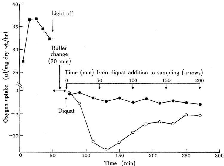
Fig. 5.—Oxygen-exchange curves for *C. vulgaris* for experiment A at 25°C. Pre-illumination at 600 f.c. in dilute carbonate-bicarbonate buffer (see text): transfer to phosphate buffer for oxygen-uptake measurements after centrifugation. ■ Control: apparent photosynthesis. ● Control: oxygen uptake after pre-illumination. ○ Oxygen uptake after pre-illumination with  $3 \times 10^{-4}$  M diquat added in darkness.
