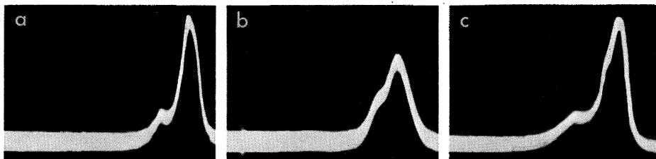
Fig. 1. Moving-boundary electrophoretic patterns (ascending boundary) of high-sulphur proteins from mouse hair at different pH values. (a) pH 4.5; (b) pH 8.6; (c) pH 11.0. Direction of movement from left to right.
