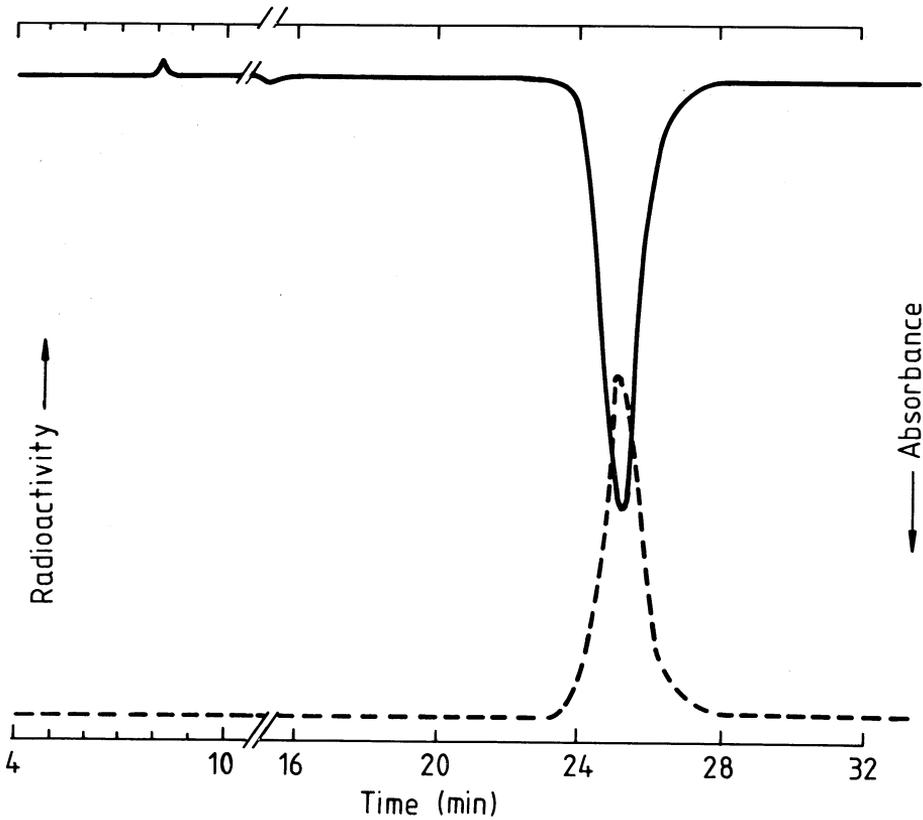
**Fig. 1.** RP IP HPLC of  $^3\text{H}$ -rm- $\alpha$ -EGF on a C-18  $\mu$ Bondapak column ( $30 \times 0.8$  cm). Mobile phase was acetonitrile-water (26:74), 0.04 M in triethylamine acetate, pH 5.6, flow rate  $1.5 \text{ ml min}^{-1}$ . UV detection at 254 nm, 0.05 AUFS (—). Radioactive detection by LSC,  $\text{dpm ml}^{-1} \times 10^{-4}$  (----).
