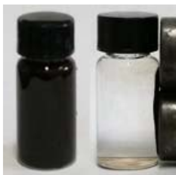
Fig. S2 Separation of DMNC by using an outer magnet.
