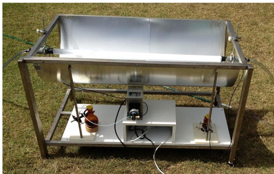
Illustration of light focusing by the trough using a red laser pointer. The capillary tube can be raised or lowered to achieve a broader or narrower focus line.
