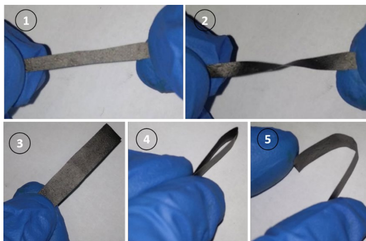
Fig. S1 Twist testing of EG/MnO 2 film electrode at different angles.
