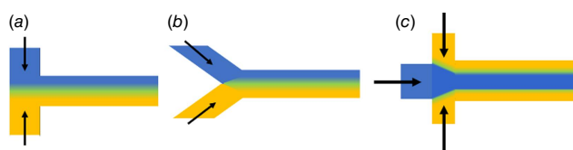
Fig. 4. Mixing of two solutions by: (a) T-junction, (b) Y-junction, (c) hydrodynamic flow focusing.
