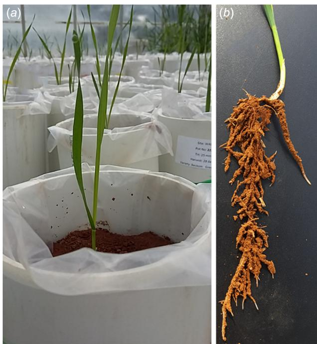
**Fig. 1.** (a) PVC tube pots (10 cm by 30 cm) packed to a bulk density of 1.3 g/cm<sup>3</sup> by placing a calculated amount of soil in each pot (~2.8 kg); pots are lined with a transparent bag to keep water in the soil. (b) Rhizosheaths adhering to roots when wheat seedlings are gently dug up.
