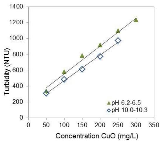
**Fig. S1.** Turbidity of CuO NPs at different concentrations and pH.
