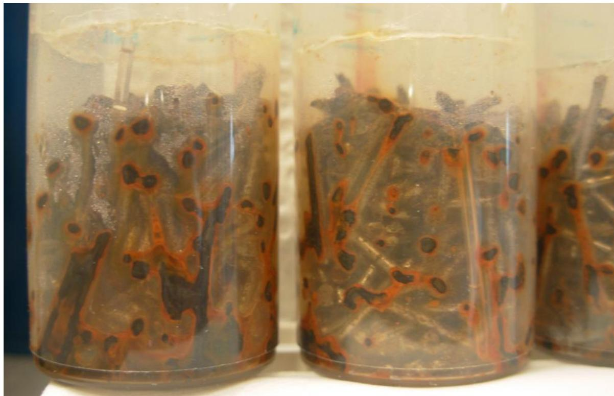
**Fig. S4.** Rusting iron nails with mostly brown Fe<sup>III</sup>-phases and black mixed Fe<sup>II</sup>-Fe<sup>III</sup> phases or magnetite.
