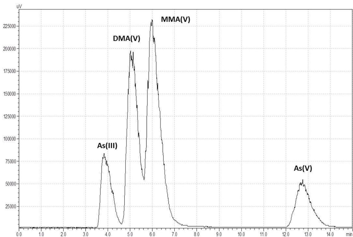
**Fig. S1.** Chromatogram of  $0.5 \text{ mg L}^{-1}$  standard solution of arsenic species  $\text{As}^{\text{III}}$ ,  $\text{DMA}^{\text{V}}$ ,  $\text{MMA}^{\text{V}}$  and  $\text{As}^{\text{V}}$ .
