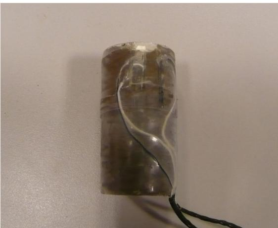
**Figure 2. The sample of Donnybrook sandstone with radial and axial strain gauges glued to its surface.**
