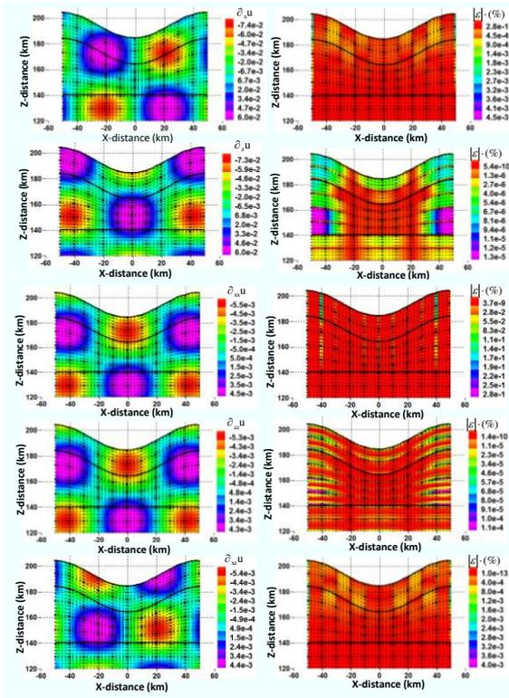
Figure 2. 2D subdomain Chebyshev differentiation results and the absolute relative errors.
