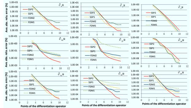
Figure 10. Convergence curves of four numerical differentiation schemes.
