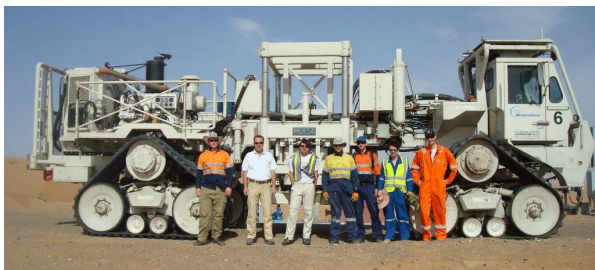
Figure 2. The 80,000 lb tracked Desert Explorer vibrator used as the source for the experiment.
