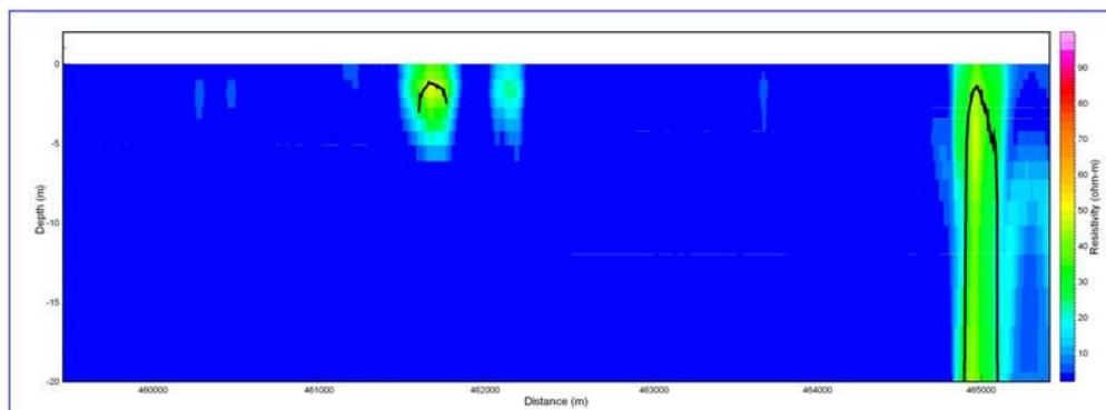
**Figure 2.** Resistivity cross-section on a ~6 km section of the proposed pipeline alignment. Depth to bedrock estimated using the statistical approach is shown as a black line. This section of line is generally very conductive and is likely to present few obstacles to excavation.
