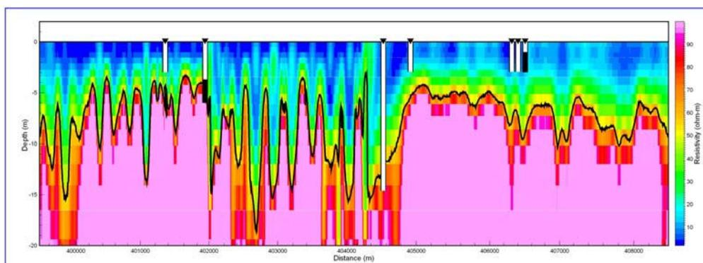
**Figure 3.** Resistivity cross-section on a ~6 km section of the proposed pipeline alignment. Depth to bedrock estimated using the statistical approach is shown as a black line. Drillhole lithology logs show unconsolidated sediments as white and crystalline bedrock as black. The depth to bedrock estimated from the AEM data is generally consistent with the drilling results and suggests that materials above a depth of 3 m will generally be excavable.
