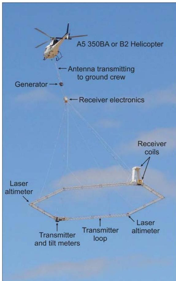
Figure 1. The SkyTEM system at a glance.
