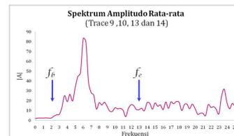
Figure 5. Average amplitude spectrum (absolute) from trace number 9, 10, 13 and 14
