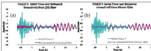
**Figure 8. The extracted ground-roll from trace number 9 in the CDP gathers data after being NMO using (a)  $(f,k)$  filter (b) Wiener filter**
