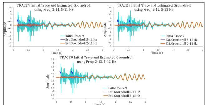
Figure 6. The extracted ground-roll of trace number 9 in the field CDP gathers data using Wiener filtering for various frequency intervals
