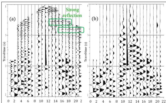
**Figure 9. The extracted ground-roll from CDP gathers data after being NMO using (a)  $(f,k)$  filter (b) Wiener filter**
