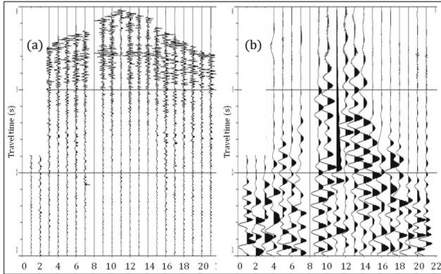
**Figure 7. Result from Wiener filtering using field CDP Gathers data with 2-13 Hz frequency interval (a) After subtracting the ground-roll from data (b) The extracted ground-roll**
