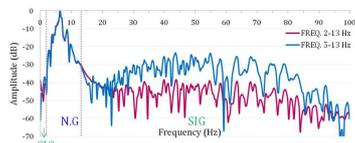
**Figure 12. Amplitude spectra (dB) of estimated ground-roll noise from Wiener filter for 2-13 Hz and 5-13 Hz in the field CDP gathers data for trace number 9**
