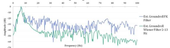
**Figure 13. Amplitude spectra (dB) of estimated ground-roll noise from  $(f,k)$  and Wiener filter in trace number 9**
