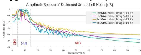
**Figure 10. Amplitude spectra (dB) of estimated ground-roll noise from four various frequency intervals in synthetic data**
