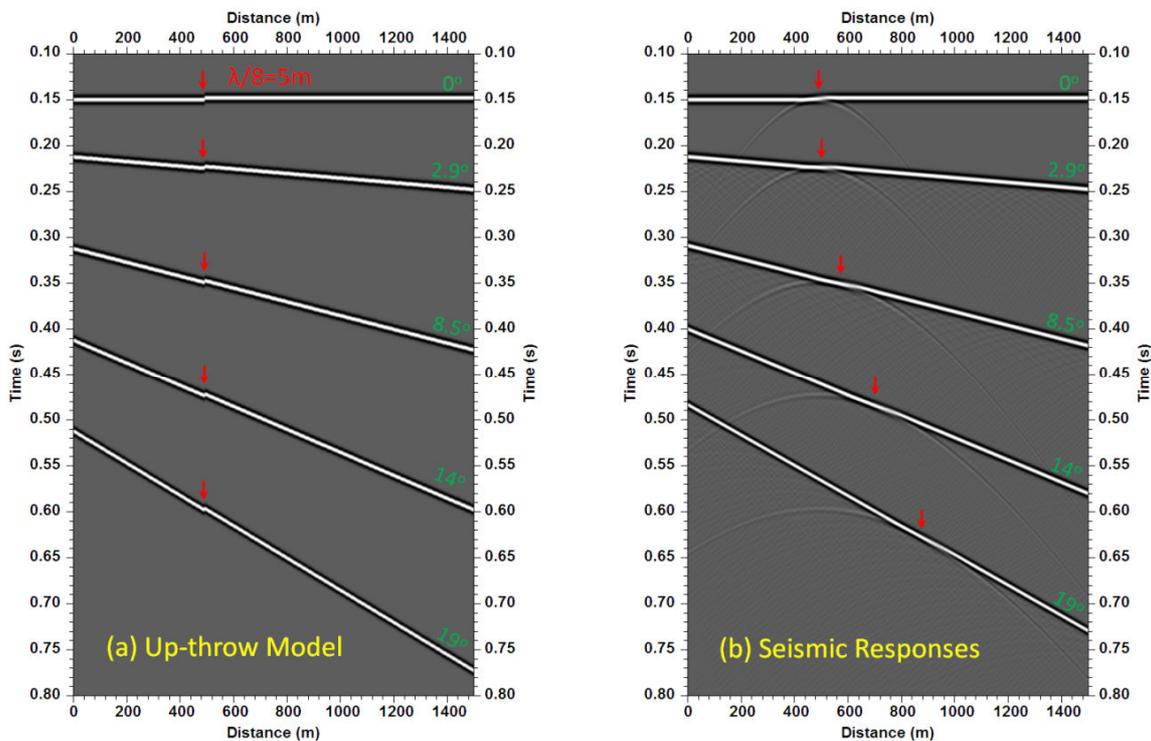
Figure 4 The effect of background structures on fault detection: (a) a 5m up-thrown fault model with dipping reflectors; (b) the seismic responses for the model in (a). A constant average velocity of 4000m/s and a Ricker wavelet with a dominant frequency of 100 Hz were used in the simulation in the F-K domain.
