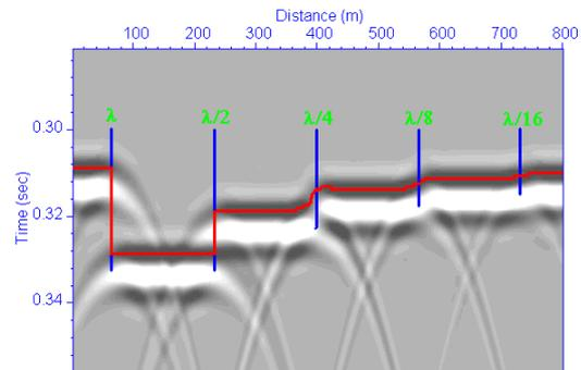
**Figure 3** The same data as shown in Figure 2 but vertically exaggerated and with accurate computer-based coal seam picks shown in red. All of the faults can be identified.
