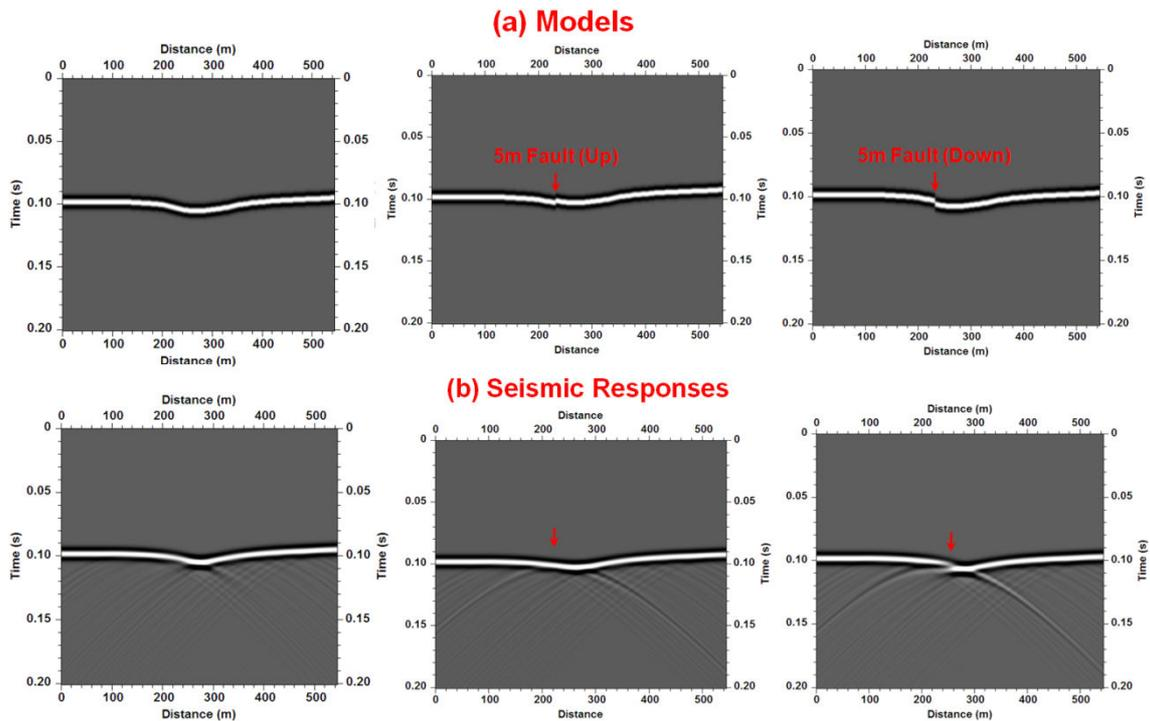
Figure 6 The effect of a syncline on fault detection: (a) fault models (Left: no fault, Middle: syncline with a 5m up-throw fault, and Right: syncline with a 5m down-throw fault); (b) the corresponding seismic responses for the models in (a). A constant average velocity of 4000m/s and a Ricker wavelet with a dominant frequency of 100 Hz were used in the simulation in the F-K domain.
