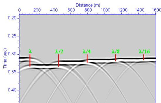
**Figure 2** A synthetic zero-offset seismic section from a reflector intersected by the faults shown in Figure 1. The sharp terminations of the faults are smeared by diffractions. The small faults are very difficult to identify visually.
