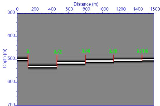
**Figure 1** A model with five vertical faults cutting through a coal seam. From left to right the fault throws are 32 m, 16 m, 8 m, 4 m and 2 m. These fault throws correspond to 1, 1/2, 1/4, 1/8 and 1/16 of the dominant wavelength.
