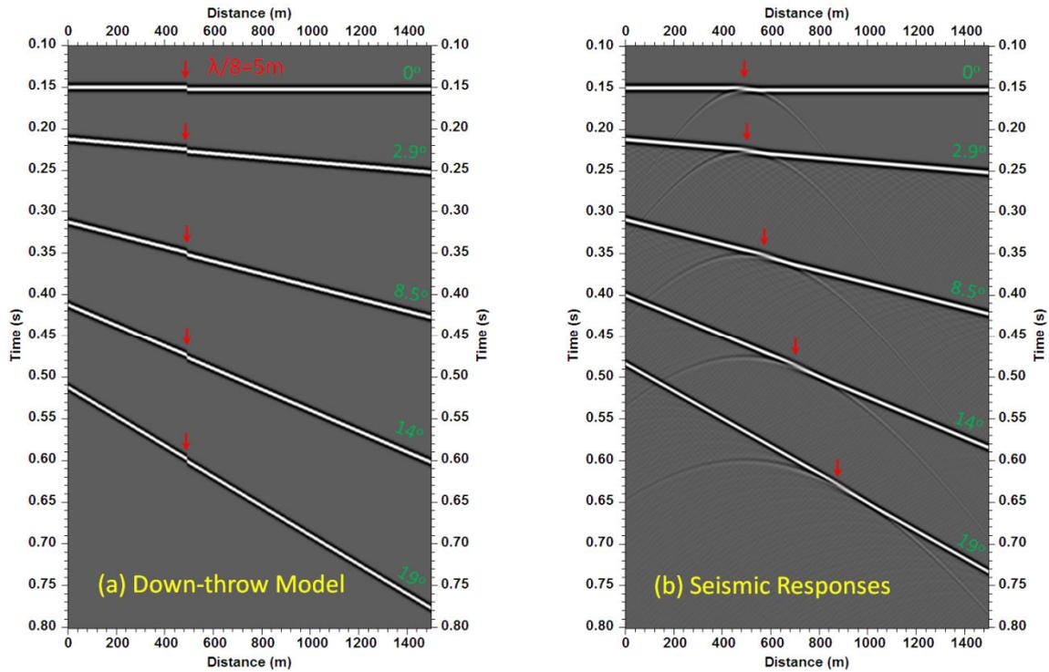
Figure 5 The effect of background structure on fault detection: (a) a 5m down-thrown fault model with dipping reflectors; (b) the seismic responses for the model in (a). A constant average velocity of 4000m/s and a Ricker wavelet with a dominant frequency of 100 Hz were used in the simulation in the F-K domain.
