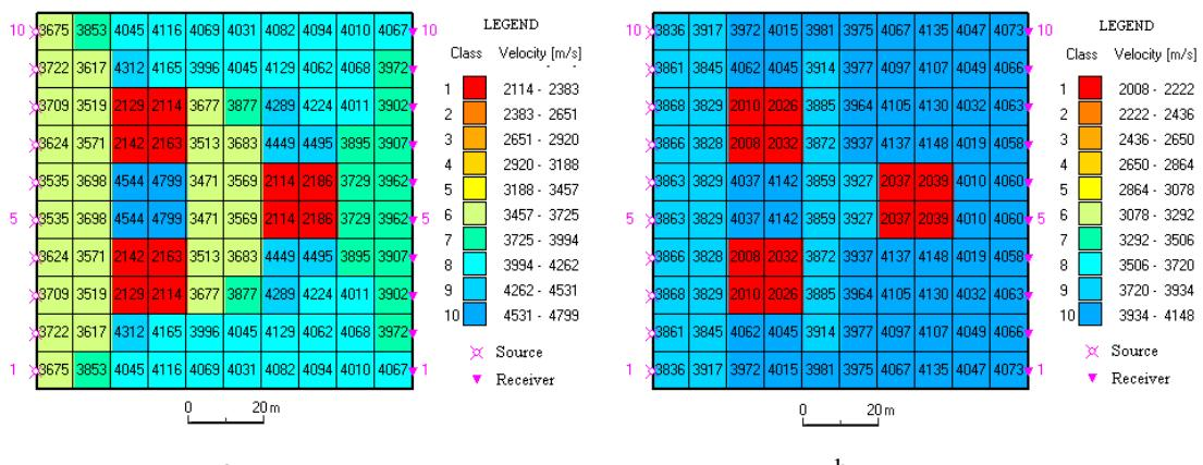
Figure 2. Tomography inversion for the model of a medium characterized by a high velocity (4000 m/s) containing three enclaves with low velocity (2000 m/s). This figure represents the results obtained by the matrix inversion method (a) and by our procedure (b) for a dataset acquired on an incomplete recording array (seismic sources and receivers on the two opposed sides of tested panel). On the upper row are depicted the velocity diagrams and on the down row the velocity maps are illustrated.
