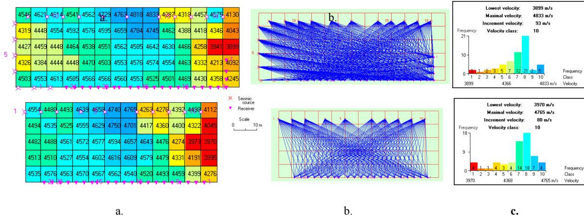
Figure 4. Velocity tomography results for a pillar situated at +240 m horizon of Prajd halite mine (100 km N. Brasov, Romania). Comparative results for the same panel in case of a quasi-complete seismic array surrounding panel (upper row), respectively simulated incomplete field array (bottom row). The columns represent: a. the plan view of the velocity distributions; b. the raypath panel coverages; c. the histograms of velocity values.
