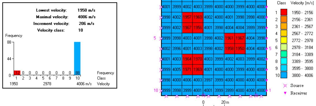
Figure 1. Tomography inversion for the model of a medium characterized by a high velocity (4000 m/s) containing three custom-defined enclaves with a low velocity (2000 m/s). This figure represents the results obtained by the matrix inversion method for a data set acquired on a recording array located completely around the panel: the histogram of velocity values (left) and the plan view of the velocity distribution (right).
