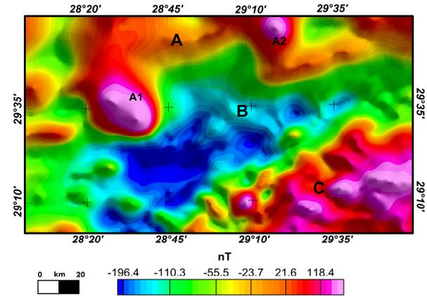
**Figure 3. Reduced to pole magnetic anomaly map of the Abu Gharadig basin. A, B, and C are regions of different magnetic patterns. Note potential anomalous basement at points A1 and A2.**
