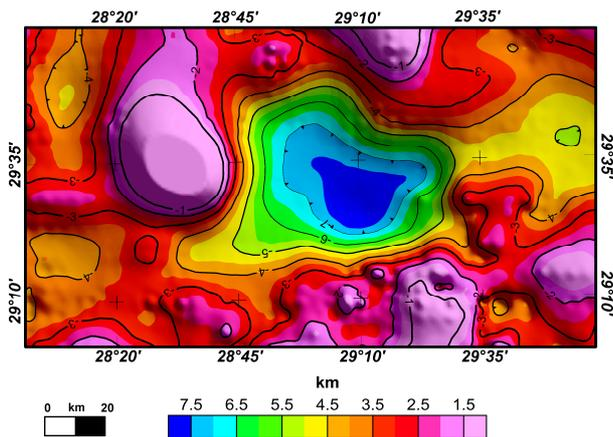
Figure 8. Depth to basement of Abu Gharadig using 3D inversion of the pseudo-gravity data.
