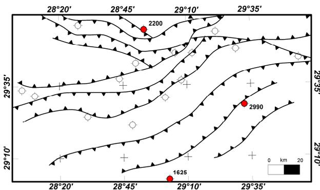
**Figure 2. Location of wells in the Abu Gharadig basin with basement depths annotated. Faults are based on the seismic interpretation of Awad (1985).**
