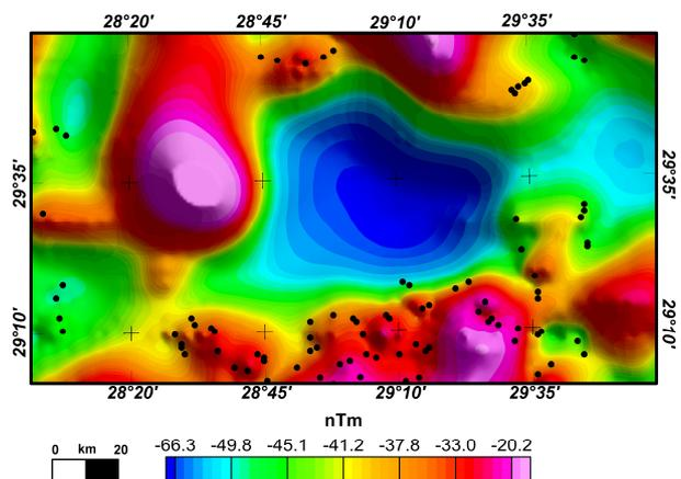
**Figure 7. Adjusted pseudo-gravity map of the Abu Gharadig basin. Circles show the control points for the inversion based on wells and Tilt-depth solutions.**
