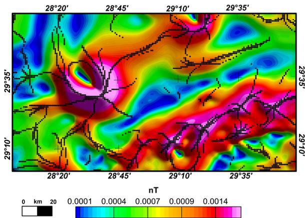
**Figure 5. Total horizontal gradient of the Pseudo-gravity of the Abu Gharadig basin. The structural trends identified by the linear maxima are highlighted by the 'ridge grid' based on the method of Blakely and Simpson (1986).**
