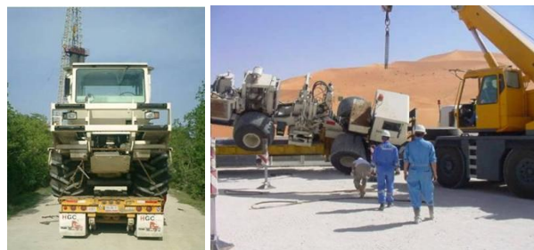
Figure 1. Examples of safety risks associated with the transport of buggy-mounted vibrators. In the image on the left the width of the buggy is greater than the trailer. In the image on the right the buggy slid off the trailer during the loading operation.
