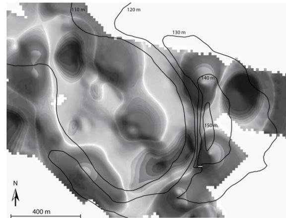
**Figure 2. High Pass filter (800m cutoff wavelength) of the Bouguer gravity data over Ecklin maar Two weak gravity highs can be observed in the centre of the maar and correlate with two magnetic anomalies.**
