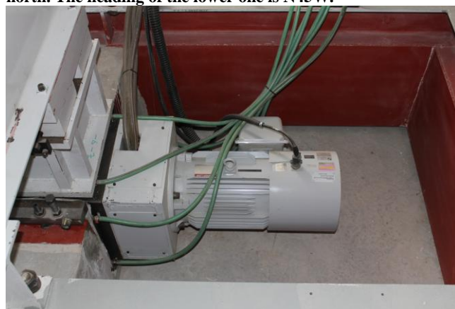
Fig. 2 Picture of the Seismic ACROSS vibrating unit showing the servo-motor.
