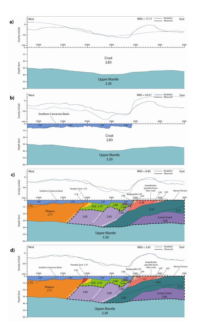
Figure 1. Forward models of the Southern Carnarvon seismic line (11GA-SC1) using the geometries outlined in the seismic interpretation of Korsch *et al.* (2013). A progression of models is shown that highlights the effect of a) the upper mantle, b) the upper mantle and Southern Carnarvon Basin, c) crustal layers and, d) crustal layers sub-divided to achieve a better fit with the observed gravity data. The extent of the Narryer Terrane is shown with a dashed black line.
