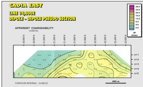
Figure 2. Dipole-dipole pseudo-section through the Cadia East mineralisation on Line 14,800 E.
