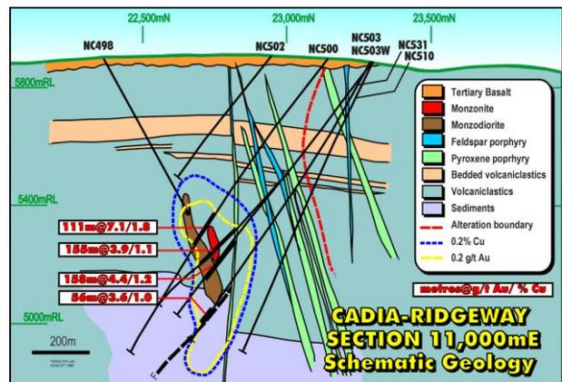
Figure 4. Schematic of Ridgeway ore body on section 11,000 E.
