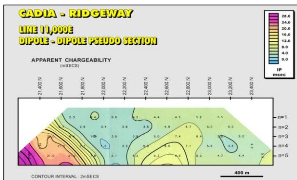
Figure 3. Dipole-dipole pseudo-section interpreted to detect the sulphide halo to the Ridgeway ore body, located 500 m below surface under 22,600 N.
