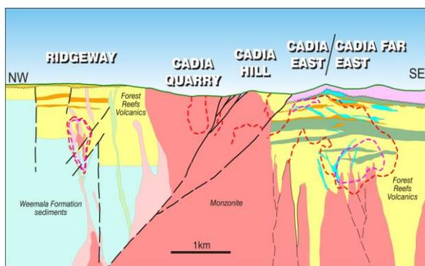
**Figure 1. Schematic long-section through the Cadia porphyry Au-Cu deposits, NSW.**
