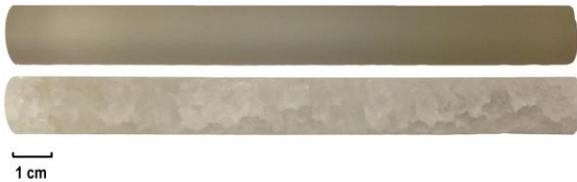
**Figure 1.** Fully dense soda-lime-silica glass rod before and after thermal cracking.
