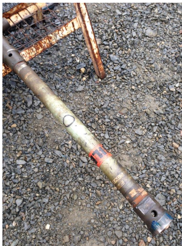
Figure 1. The Shuttle after field testing at DET CRC research facility in Brukunga, South Australia. This tool is inserted between the back-end assembly and inner core-tube. Outer tube sub units of equivalent length are inserted in the drill-string BHA prior to drilling to keep the core latching mechanisms in their proper place.
