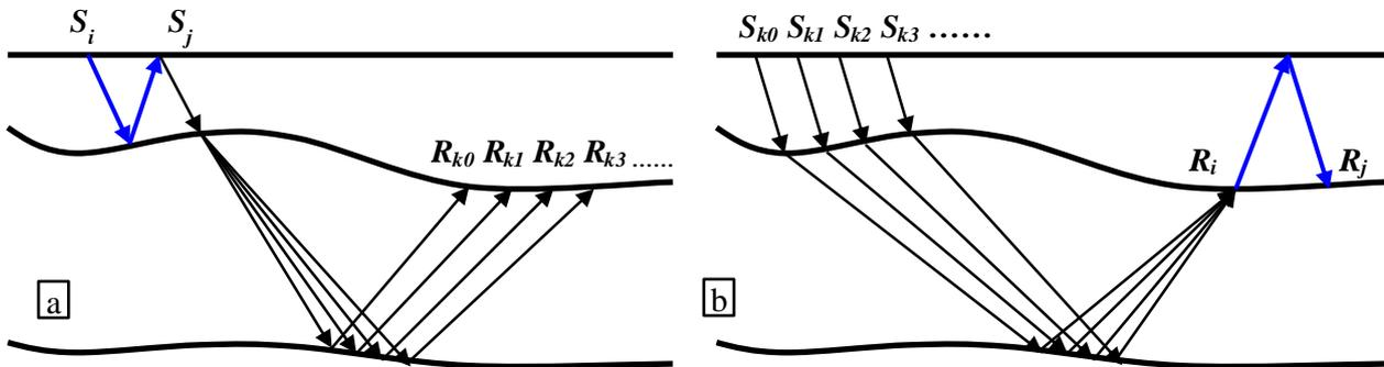
Figure 2 (a) Interferometry obtaining the Green's function  $S_i S_j$  (blue arrow) to predict OBC shot side surface related multiples (b) Receiver side illustration.
