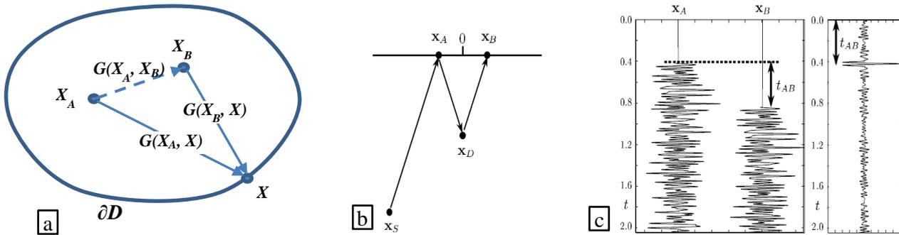
Figure 1 (a) Green's function  $G(X_A, X_B)$  can be obtained by cross-correlating observations at  $X_A$  and  $X_B$  by integrating sources  $X$  along  $\partial D$ . (b) Half plane 1D illustration of random source  $X_S$ , scatterer  $X_D$ , and two receivers at  $X_A$  and  $X_B$ , (c) Observations of a random source at  $X_A$ ,  $X_B$  and their cross-correlation, which gives the reflection response.(Wapenaar et al. 2004, 2006)
