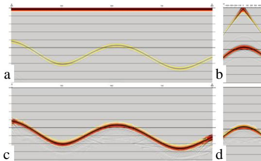
Figure 4 (a) Numerically simulated zero offset streamer data. (b) Shot gather of streamer data. (c) Zero offset section from OBC data interferometry. (d) Shot gather from interferometry.
