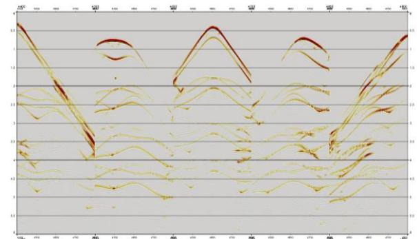
Figure 5. Predicted multiple model using OBC data only, shot and receiver side operators generated from interferometry, with prediction method similar to that in SRME by convolve data with operators.
