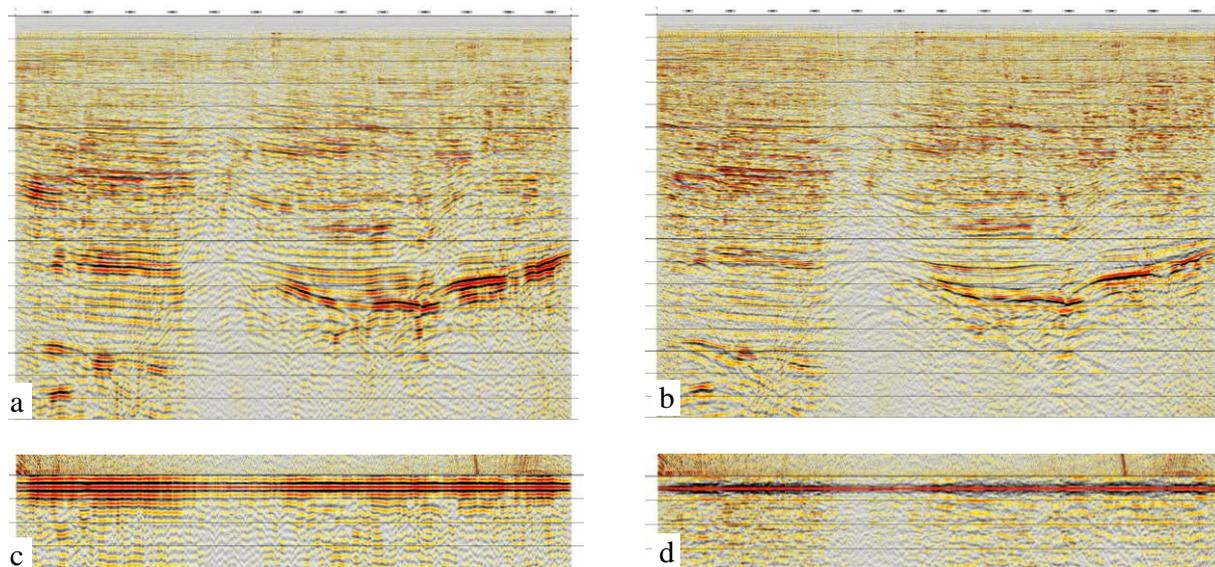
**Figure 6, (a) P-wave stack after noise and ghost removal but before demultiple, (b) demultiple stack using our method, (c) autocorrelation before demultiple, (d) auto correlation after demultiple**
