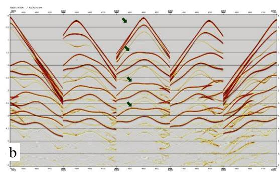
Figure 3, (a) Synthetic velocity model with four primary events; the dashed line highlights the water bottom. (b) Numerical P-wave seismic response including surface related multiples.
