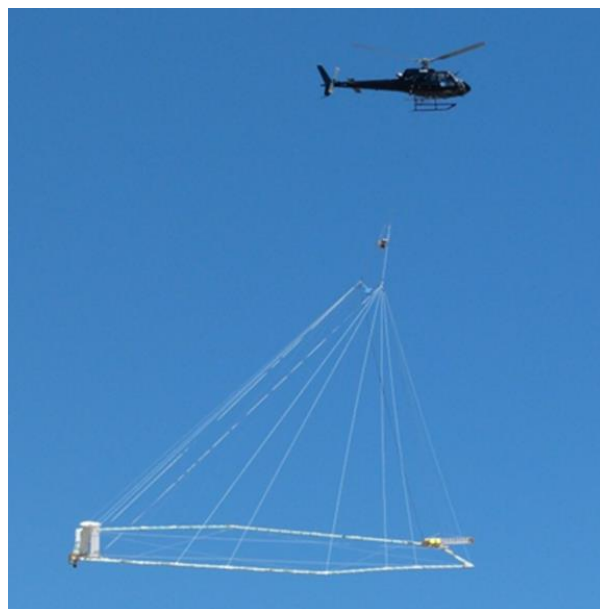
Figure 2. SkyTEM airborne EM system in operational mode.
