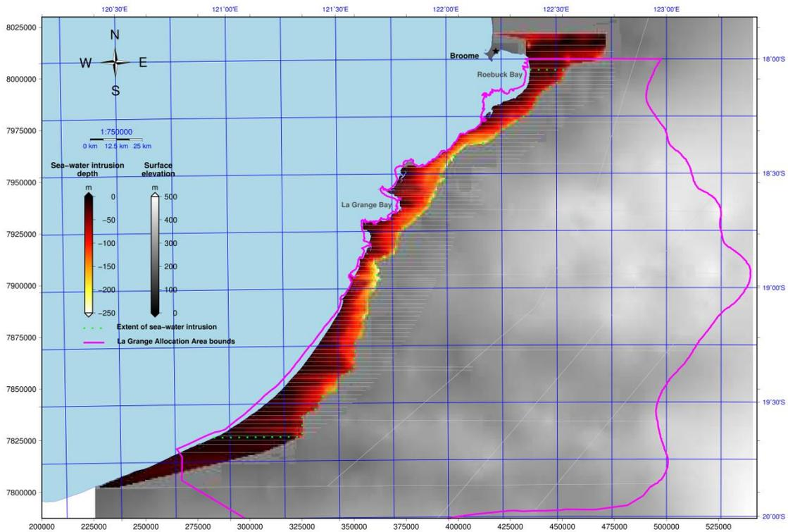
**Figure 3 Variation of salt-water intrusion distance and depth. Distance is given by the spatial extent of the colours, and depth is given by colour variation. The dashed green line indicates confidence of interpretation of sea-water intrusion. The magenta line marks the extent of the La Grange Allocation Area. The underlying gray scale image plots surface topography.**
