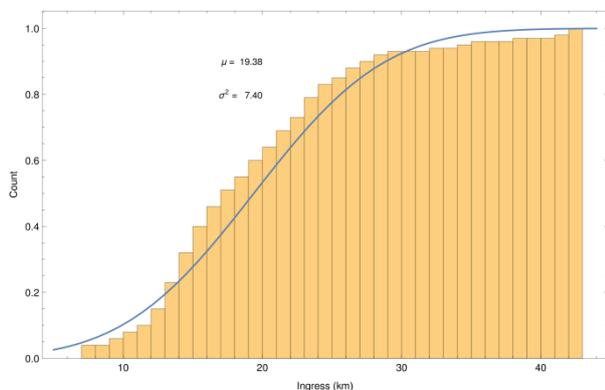
**Figure 4 Distribution of distance of maximum salt water ingress. This distribution is compared to that of a normal distribution having the same mean and standard deviation.**
