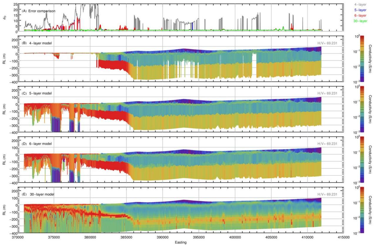
**Figure 2 Comparison between blocky and smooth model inversions and their error for Line 1004301. Errors are compared in Panel A. Blocky model inversions are shown in Panels B, C and D (four, five and six layer); smooth model inversion results are shown in Panel E. Five-layered blocky models are generally preferred because of their parsimonious balance between low errors, geological accuracy and model parameterisation.**
