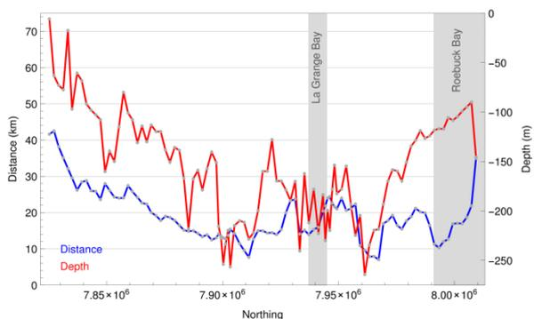
**Figure 5 Comparison of depth to sea water at its easternmost extent with ingress distance. Distance is plotted against the left axis while depth is plotted against the right axis.**
