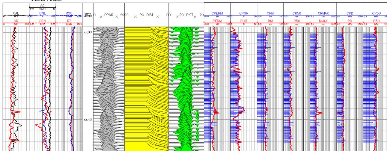
Figure 9: A field example of evaluating formation pore structure from pseudo  $P_c$  curves in tight gas sandstone reservoirs.
