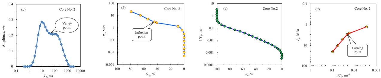
Figure 4: The relationships of  $1/T_2$  versus  $P_c$  for core No.2 with typical bimodal NMR spectrum.
