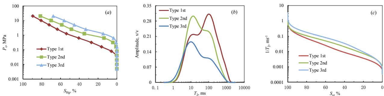
**Figure 7: Three types of average MICP curves, NMR spectra and the corresponding NMR reverse cumulative curves.**
