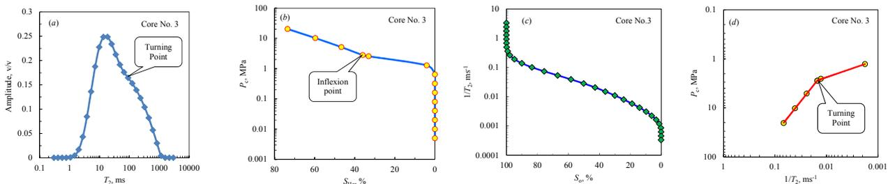
Figure 5: The relationships of  $1/T_2$  versus  $P_c$  for core No.3 with non-typical bimodal NMR spectrum.
