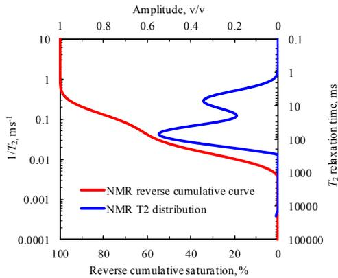
**Figure 1: Principle of acquiring NMR reverse cumulative curve from NMR  $T_2$  distribution**
