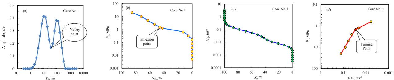
**Figure 3: The relationships of  $1/T_2$  versus  $P_c$  for core No.1 with typical bimodal NMR spectrum.**
