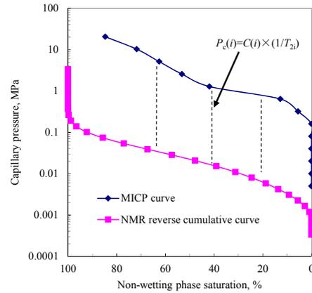
**Figure 2: Principle of obtaining optimal C from NMR logs.**
