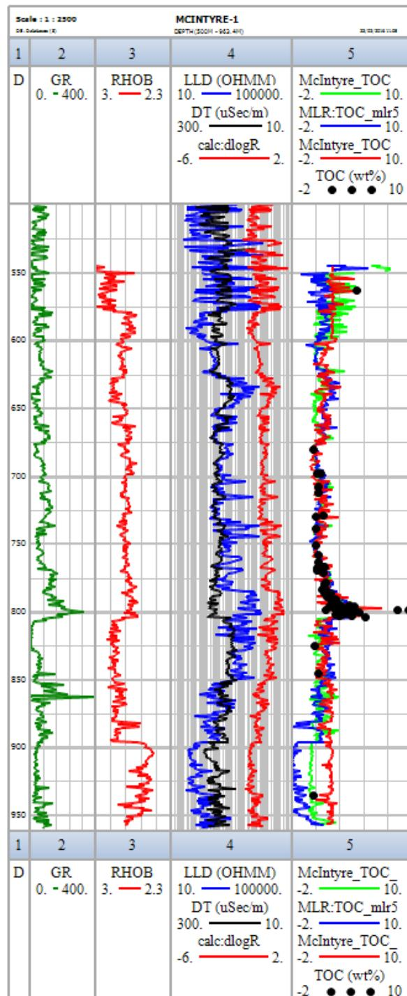
Figure 3: McIntyre-1 logs and TOC predictions: (1) depth, (2) GR, (3) RHOB, (4) logLLD and DT separation and  $\Delta \log R$ , and (5) core TOC in comparison with MLR, MLP and SVM predictions.
