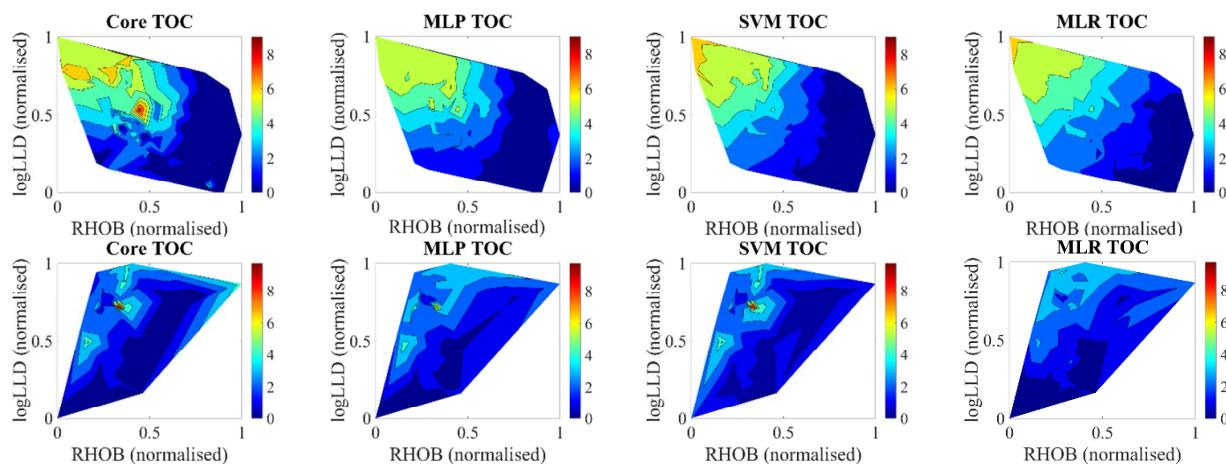
**Figure 2: Core TOC contours for normalized RHOB and logLLD at Altree-2 (top row) and McIntyre-1 (bottom row) compared to TOC contours from MLP, SVM and MLR models. The Altree-2 MLP TOC and McIntyre-1 SVM TOC contours are most similar to those for the core TOC. The MLR TOC contours are much smoother, missing significant detail in comparison with the nonlinear models.**
