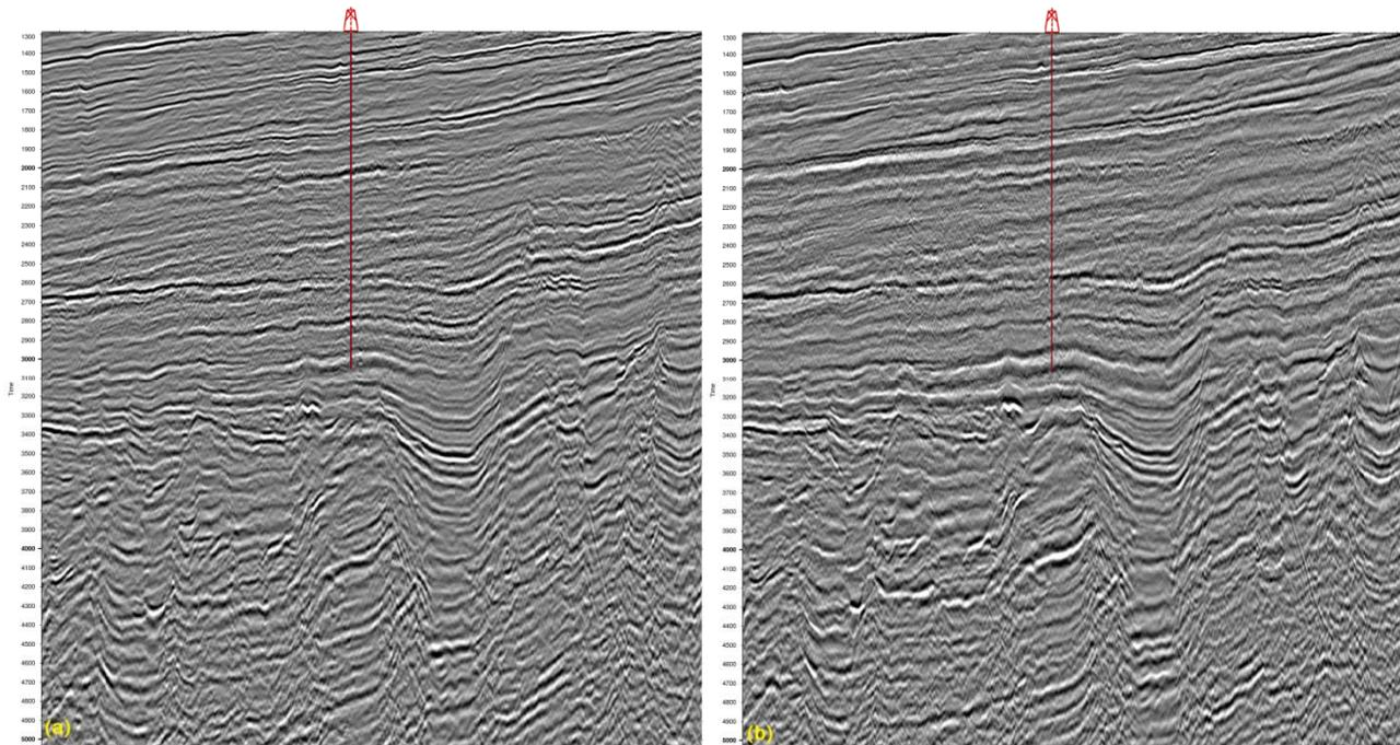
**Figure 6: Comparison between the vintage processed stack (a) and the current reprocessed stack (b), with the Brewster-1A well overlaid.**
