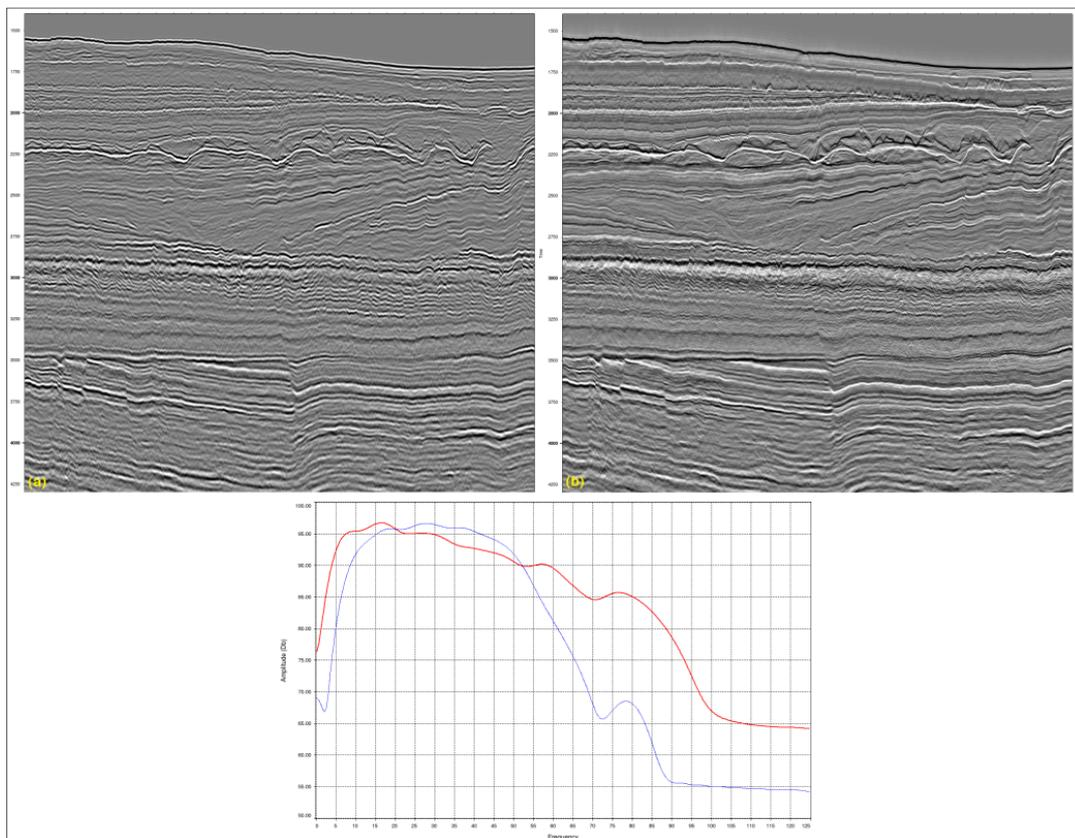
**Figure 3: Comparison of the north-west portion of the survey line, where (a) is the vintage processed stack and (b) is the current reprocessed stack. There is an overall broader frequency range on the current reprocessed stack which could assist interpretation, particularly around the pinchout structures at ~3500ms. The amplitude spectrum for this section is also shown where the thin blue curve is the vintage processed dataset and the thicker red curve is the current reprocessed dataset.**
