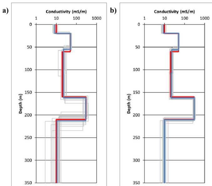
Figure 3 Forward model (red), each noise perturbed inverted model (grey), and average inverted model (blue); using a) standard Tempest noise model, b) High Moment Tempest noise model.
