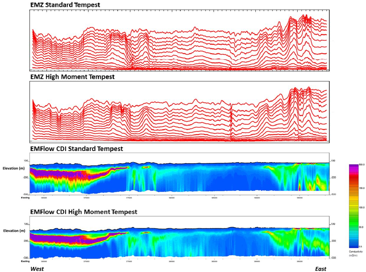
Figure 4 EMZ data and EMFlow CDI for a test line located near Gingin, WA, flown with standard and High Moment Tempest.
