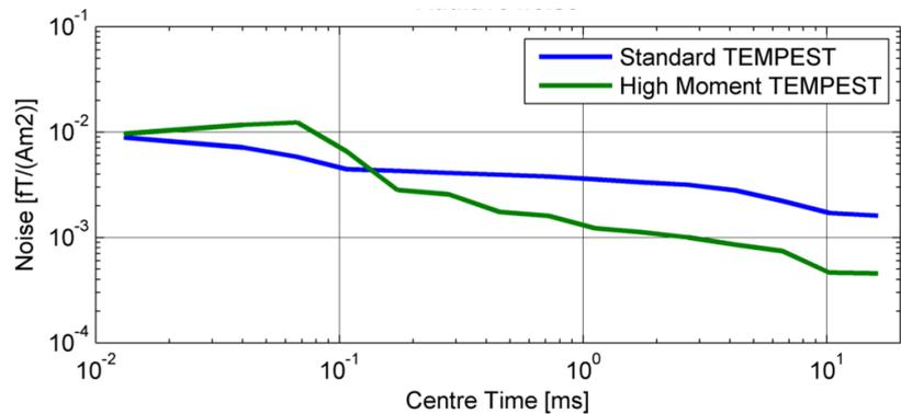
Figure 2 Additive noise (standard deviation of signal at high altitude) for standard (blue) and High Moment Tempest (green).
